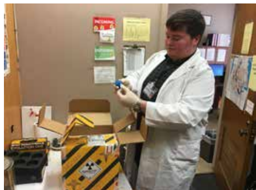
RSO Technical Assistant Kyle Huber checks in a White-I radioactive package containing tin-117m for metastatic bone disease treatment.
