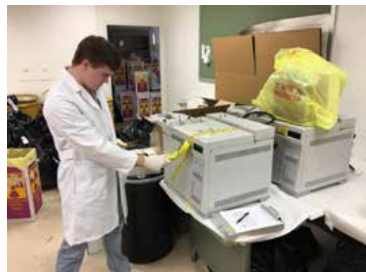
RSO Technical Assistant Blaine Irle performs a radioactive contamination survey on gas chromatography equipment.
