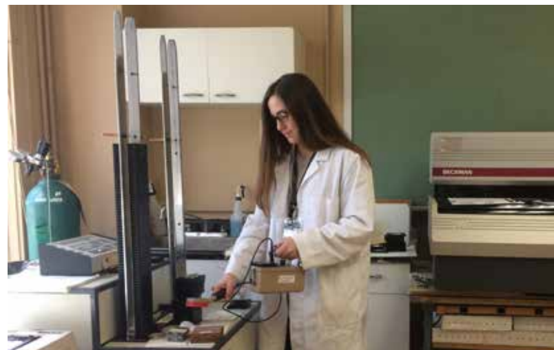
RSO Technical Assistant Caroline Babin performs a routine survey of a radioanalytical laboratory using a Geiger Müller meter.
