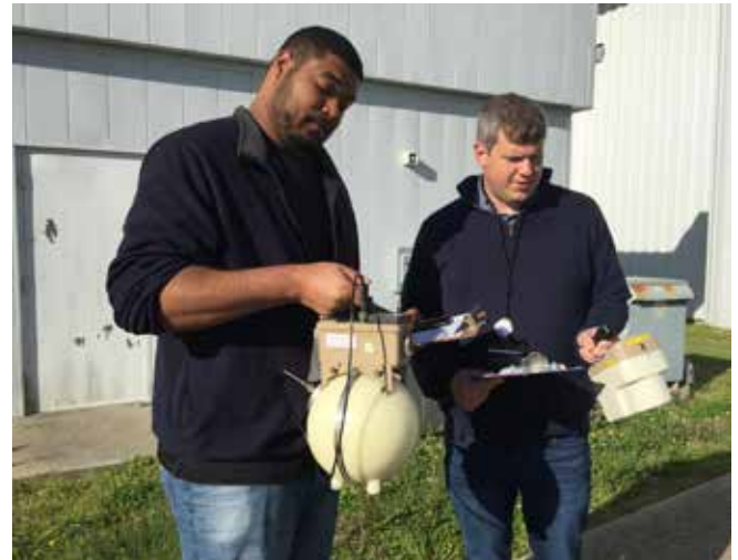
LSU environmental health physics graduate student from the Department of Environmental Sciences Nicholas T. Desselles (left), supervised by CAMD Radiation Safety Officer Charles A. Wilson IV (right), uses different types of radiation detection equipment (i.e., a neutron survey meter and a pressurized ion chamber meter) to measure ambient radiation levels at CAMD for his master's research project.
