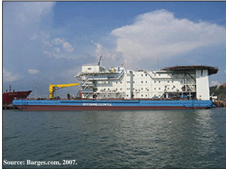
Figure 41. Offshore floating accommodations (Floatel).
