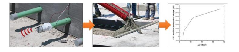
The Al-guided real-time concrete sensing system.
