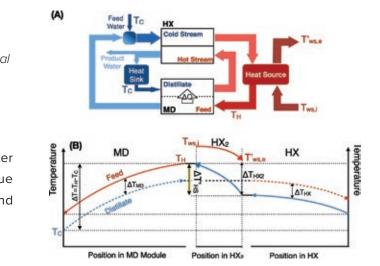
Figure 4 – (A) Schematic and (B) temperature profiles for a countercurrent direct-contact membrane distillation (DCMD) system with recycled feed and distillate streams and a heat exchanger to recover heat from the distillate stream and another heat exchanger to harness heat from a waste-heat source.
