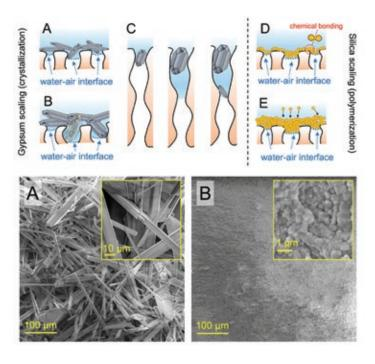
*Figure 1 – Schematic illustration of the scalant growth* process on porous membrane substrates during separation of high-salinity feed solutions saturated with gypsum (left) or silica (right).
