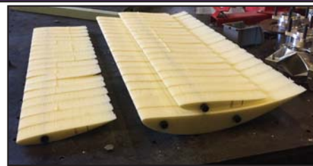
Foam core with carbon spars
