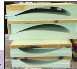
Foam core with carbon spars
