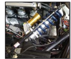
Sensors to data log shock travel
