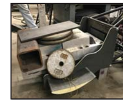
Initial front wing mount loading to failure
