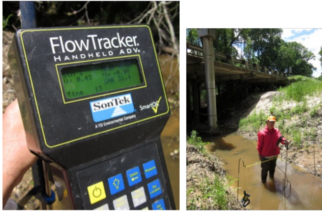
Figure 10. LGS staff conducting a Flow Tracker survey of Shettleworth Bayou near Shreveport, Louisiana on April 30, 2014, image on right is a close up view of the Flow Tracker in operation for survey of Shettleworth Bayou on April 30, 2014.
