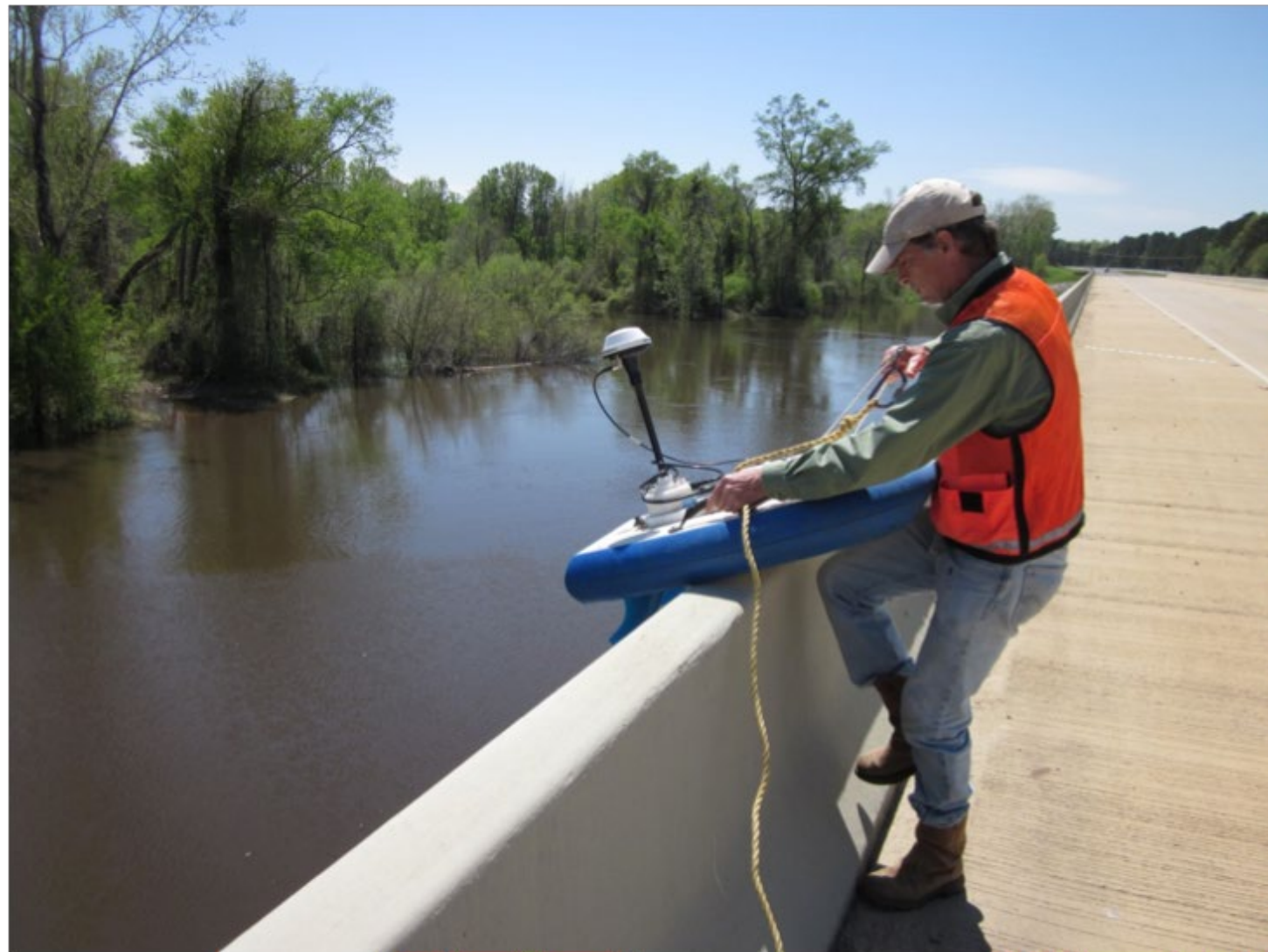
Figure 7. LGS staff getting ready to place River Surveyor over the edge of the bridge to start survey of Little River near Rochelle, Louisiana on April 4, 2014.
