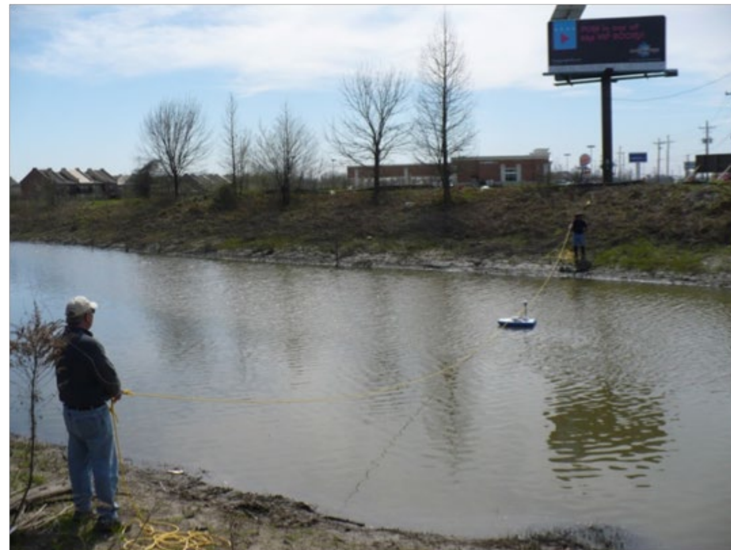
Figure 5. LGS staff measuring stream discharge for Bayou Fountain at Bluebonnet Boulevard in Baton Rouge on March 7, 2013.
