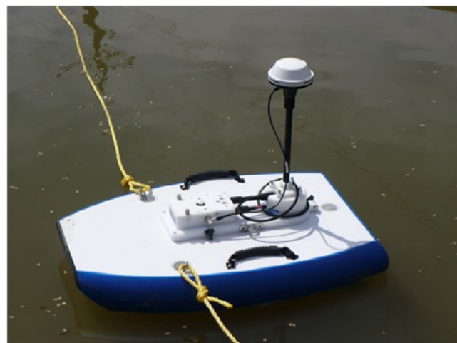
Figure 4. A close up view of the River Surveyor. Box towards bow end (left) is power source, the tower near stern (right) is global positioning system (GPS) unit used for locating boat on universal grids (latitude-longitude or State Plan Coordinates (UTM)).
