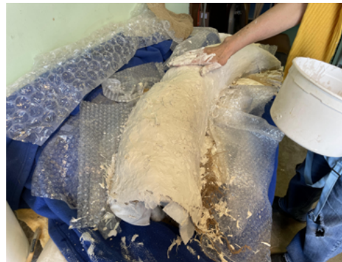
Fig. 6 Left: Dr. Suyin Ting adds plaster and shredded packing stuffing to the plaster cast.
