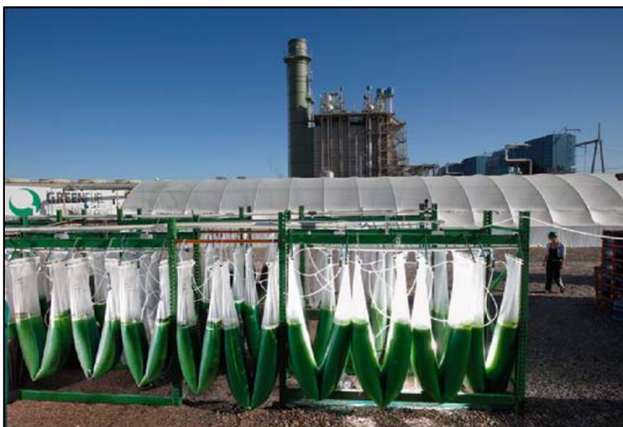
Figure 19 Algae Production from Power Plant Exhaust (Borne, 2007)
