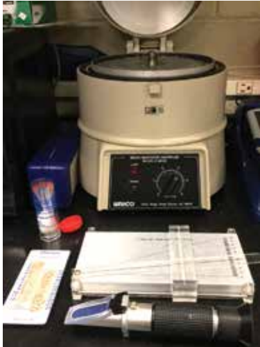
Fig 1: Centrifuge, micro-hematocrit tubes, hematocrit reader, and refractometer used to determine PCV and TS measurements.
